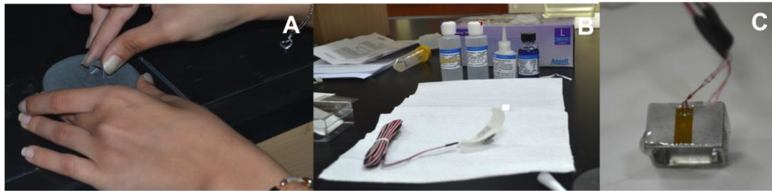
Fig. 4 A , each bite block was ground with increasingly fine abrasive papers to smoothen the surfaces. B , bonding of the strain gauges to the sides of the frame. C , insulating the block with a layer of clear epoxy resin.
